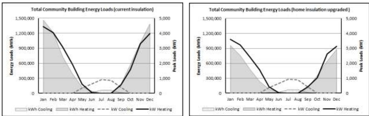
a) **Figure 1** (a) This graph illustrates the total building heating and cooling energy loads with the existing homes as they are currently insulated. (b) This graph illustrates the total building heating and cooling energy loads, but with upgraded insulation standards in the homes.
